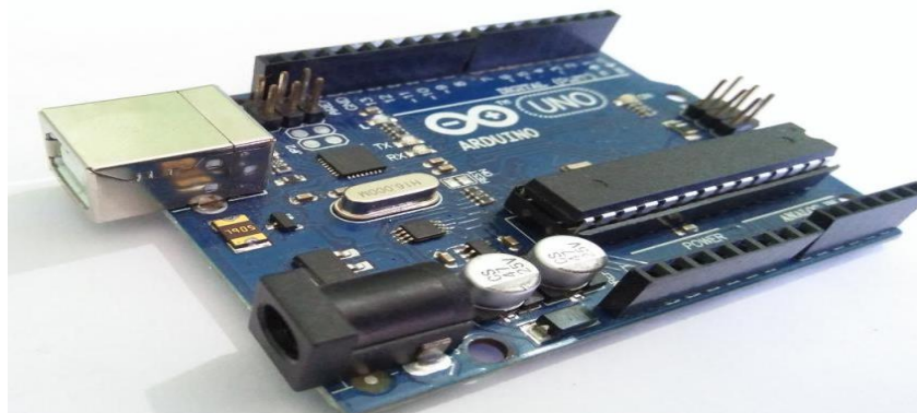
FIG.1 Arduino hardware structure
